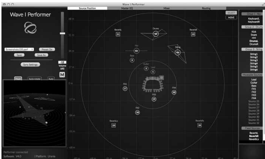
Figure 6.49 – WavePerformer, outil de visualisation/manipulation des sources virtuelles en exploitation, © Sonic Emotion.
