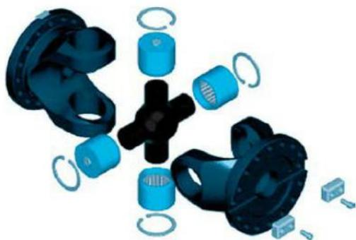
Figure 7.5 Joint de cardan simple.
