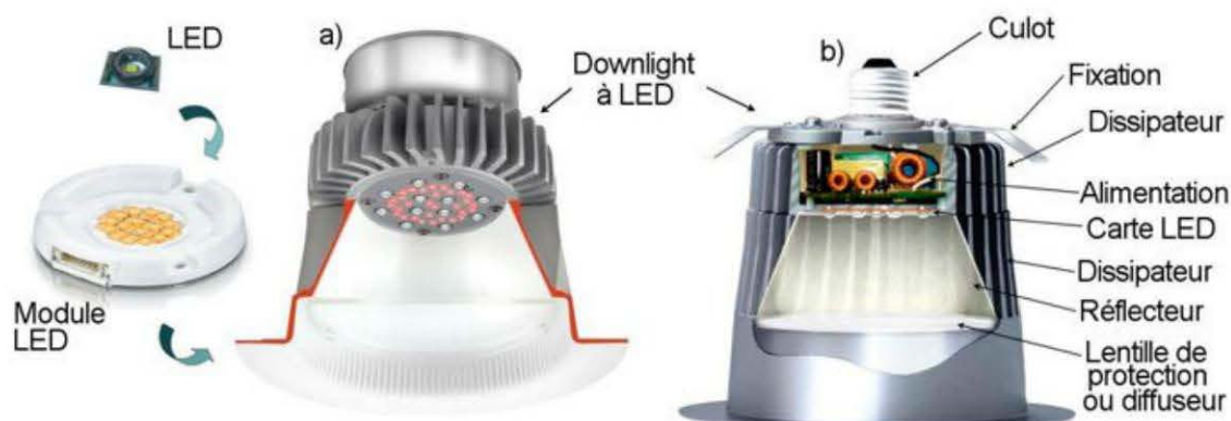
Figure 10.21 – Down light utilisant un module LED (a = Thorn, b = CREE).
