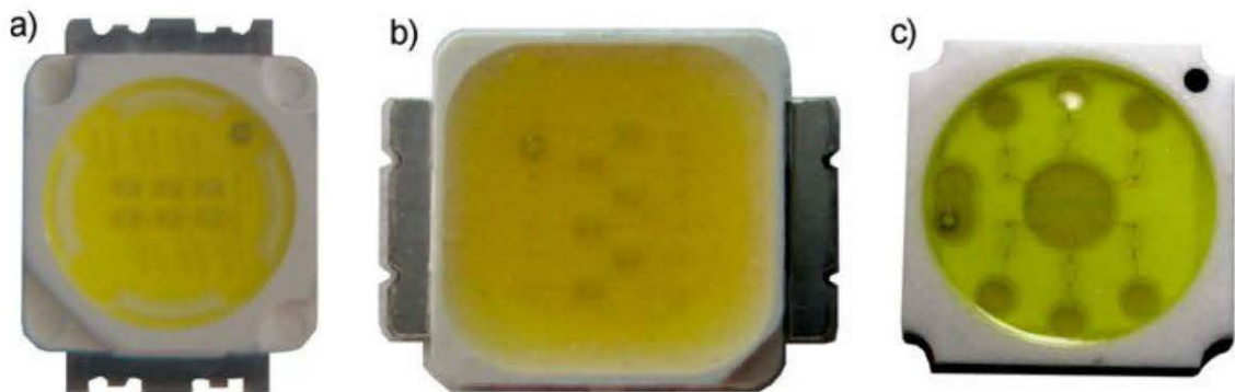
Figure 9.18 – LED multi-puces (a = Nichia ; b = CREE ; c = Stanley).
